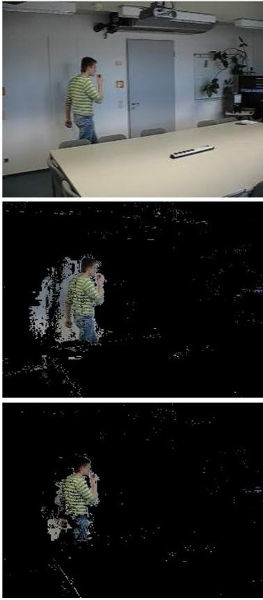
**Figure 3. Detection of foreground in an input image (top) using only background detection (center) and background detection in combination with shadow detection (bottom). Only non-black pixels are considered foreground.**
