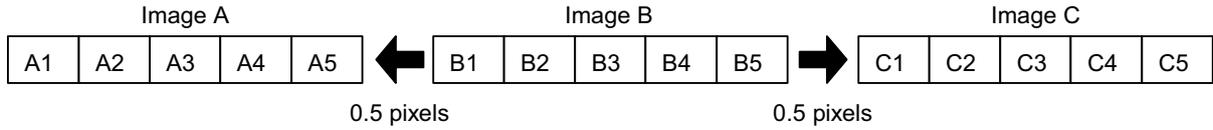
**Figure 2. One dimensional model of input images**
