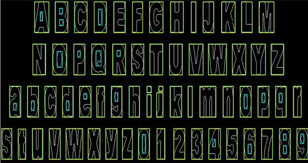
**Figure 2. Edge-boxes for the English alphabet and numerals. Note that there is no character that completely encloses more than two edge components**
