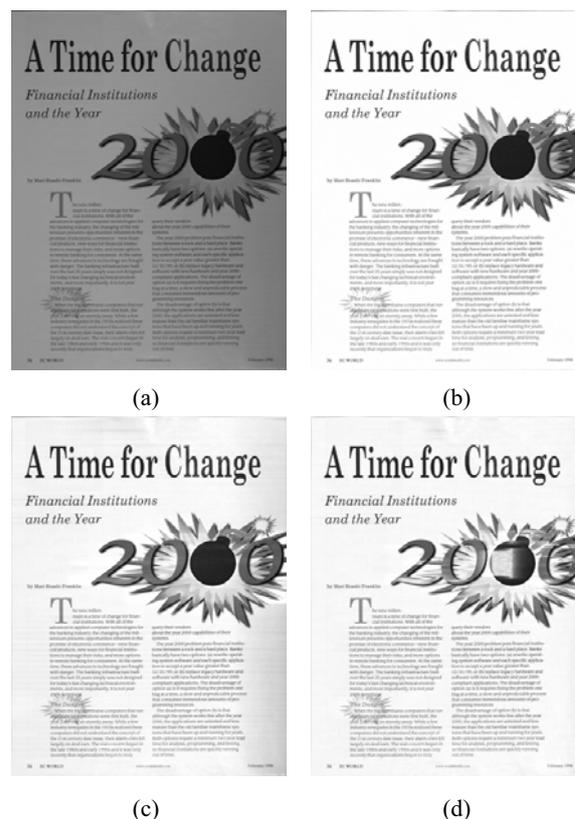
Figure 8. Comparison with Hsia *et al*'s method. (a) grayscale version of the image of Figure 4 (a); (b) illumination corrected using the proposed method; (c) correction with Hsia's method, with  $N = 5$ ; (d) correction with Hsia's method, with  $N = 10$ .
