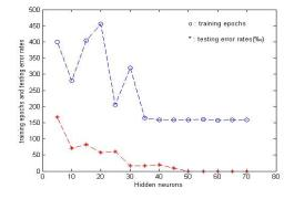
Figure 7. Epochs trend and testing errors against number of hidden neurons
