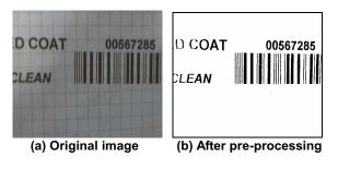
Figure 2. Captured garment barcode label and its pre-processing result
