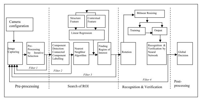
Figure 1. Schematic construction of the automatic digit location and recognition system
