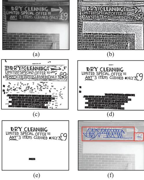
**Figure 4. Steps of the text segmentation and grouping. (a) Original image, (b) Adaptive threshold, (c)–(e) result after filtering by size, border energy and Eigen-transform measure, (f) perceptual grouping.**
