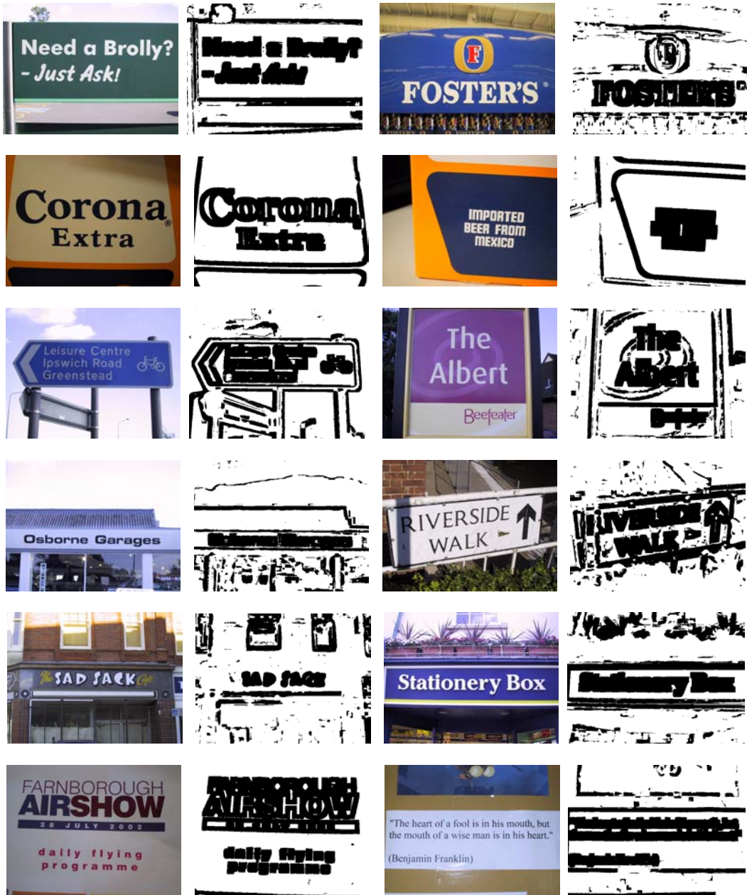
Figure 6. Text detection examples (test database) Text detector: neural classifier with window size 17x17
