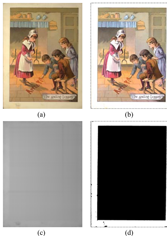
Figure 5. A figure-only book page. (a) cropped image (2409×3224) for enhancement; (b) enhanced image with the proposed method; (c) estimated illumination surface; (d) segmentation map.
