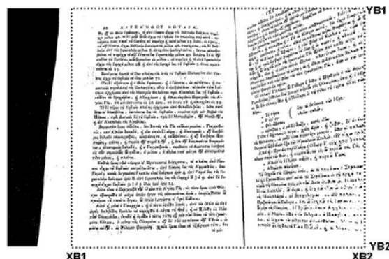
Figure 3. Limits XB1, XB2, YB1 and YB2 of text regions after noisy black border detection.
