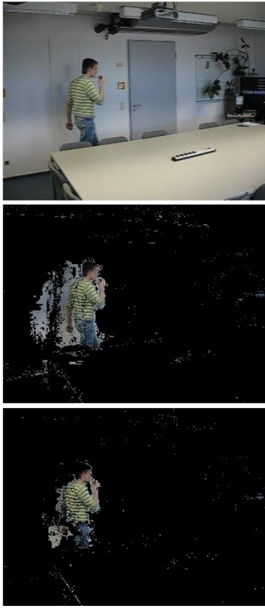
Figure 3. Detection of foreground in an input image (top) using only background detection (center) and background detection in combination with shadow detection (bottom). Only non-black pixels are considered foreground.
