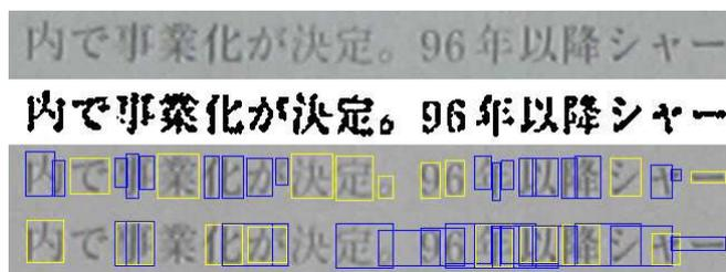
Figure 1: Segmentation of degraded text string.
